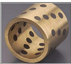
The product is based on a special formula alloy copper, inlaid with a special formula of solid lubricants, solid lubricant friction area of more than 20%. This copper alloy and non-metallic anti-wear materials advantages, break the limit of the general bearing to rely on the boundaries of oil film lubrication, achieving oil-free lubrication. It can be widely used in metallurgy, rolling equipment, ore machinery, boat machinery, steam turbines and so on.
