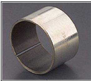
The product uses steel plate as the base, the middle is sintered spherical bronze powder, the surface is rolled polytetrafluoroethylene (PTFE) and lead mixture, made by the rolling bearing. With a small coefficient of friction, wear resistance, good corrosion resistance and no oil lubrication characteristics.
