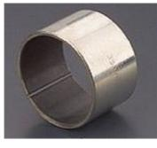
The product uses steel plate as the base, the middle is sintered spherical bronze powder, the surface is rolled polytetrafluoroethylene (PTFE) and lead mixture, made by the rolling bearing. With a small coefficient of friction, wear resistance, good corrosion resistance and no oil lubrication characteristics.
